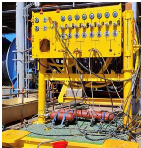
Figure 3—Photo of Retrofit RWOCS Panel Bladder-Accumulator Skid
