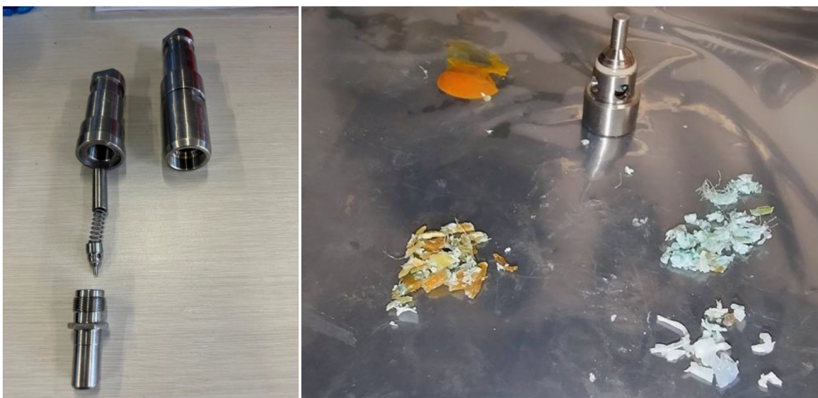
Figure 4—(a) Assembled and Disassembled Poppeted Coupler; (b) Poppet from Blocked Connector with Blockage Material Separated by Type
