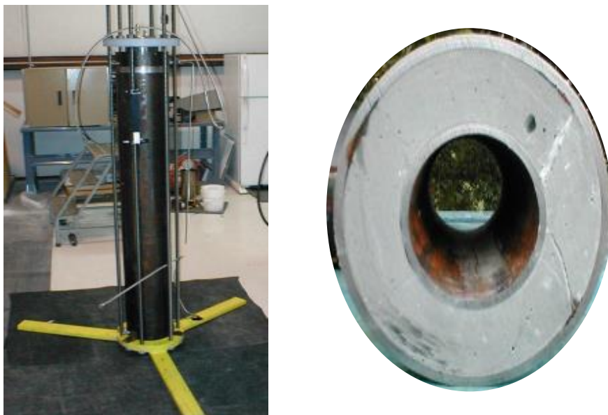
Figure 2. Microannulus Test Fixture and Cross Section from Rusch and Slezak, 2005
