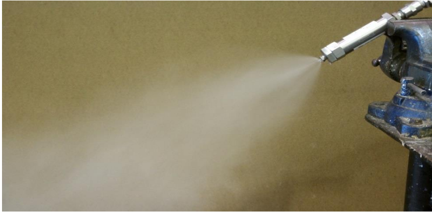
Figure 5: Misting Nozzle Atomizing Sealant
