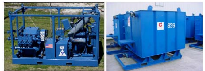
Figure 3b. Triplex pump and blend tank in the second case history
