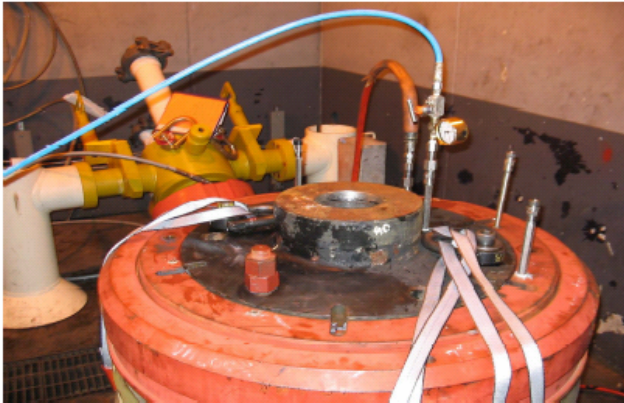
Figure 1. Sealant efficiency test on a flowline hub
