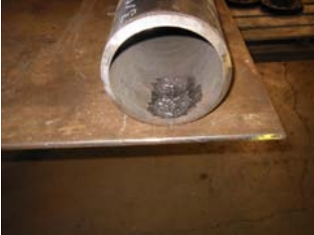
Figure 8: Overview of Internal Corrosion Defect Section
