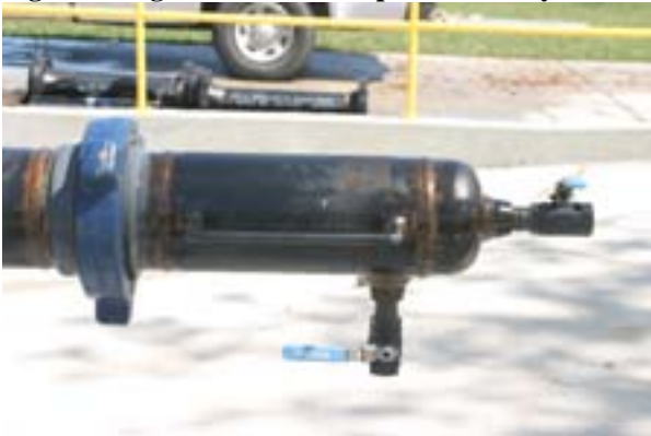
Figure 4: Pig Launcher / Receptor Assembly
