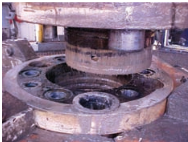
在节流管线的连接处可能会发生泄漏 Leaks can occur at choke line connections
