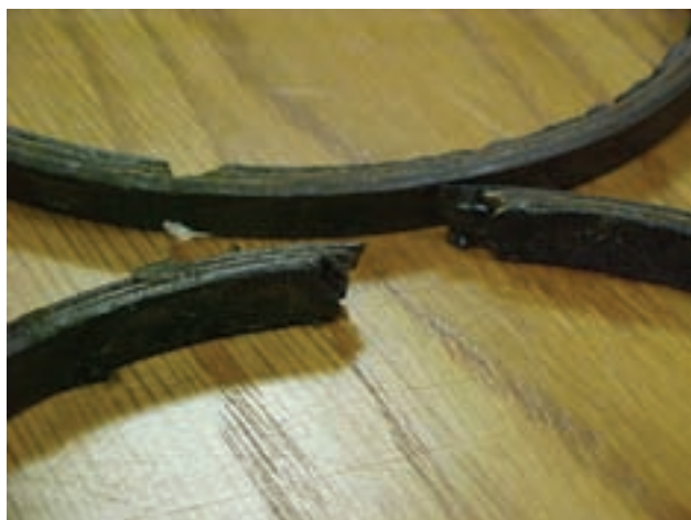
节流管线密封口的损坏会导致泄漏 Damage to choke line seals creates leaks
