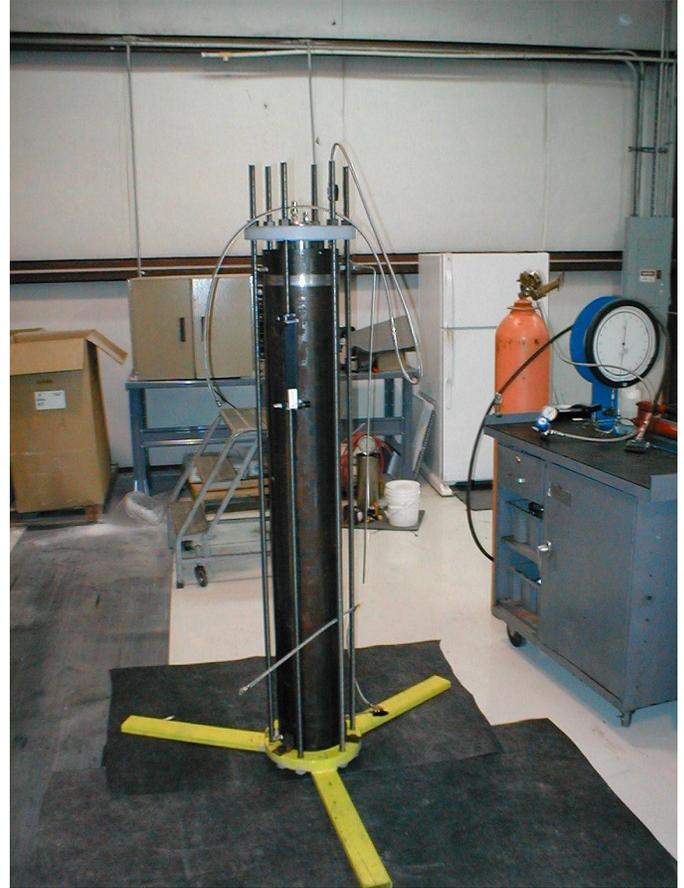
Cement was pumped into the annular space of the test fixture between the inner and outer casing strings. While the cement was curing, pressure was maintained in the inner string. Once the cement is cured, the inner casing pressure was released, creating an annular void space between the inner casing and the cement sheath. The release of pressure resulted in the creation of cracks and fissures in the cement.
