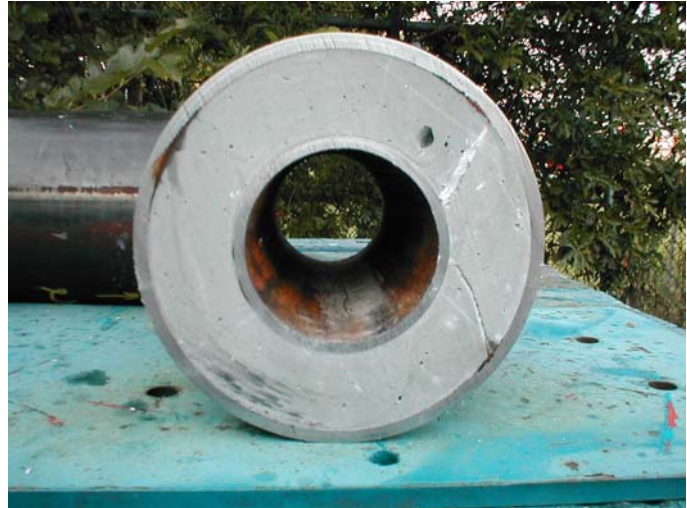
Figure 2: Annular Cross-Section – Test Fixture
